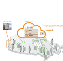
A SAMPLING OF COLLECTED PARAMETERS Base Stations: Operator, nodeB ID, radio type, TAC,... Channels: Frequency, PCI, bandwidth, online, stand alone, TDD frame structure... Dynamic RF (per channel): Signal power, RSRP, RSRQ, SINR, Occupancy...
