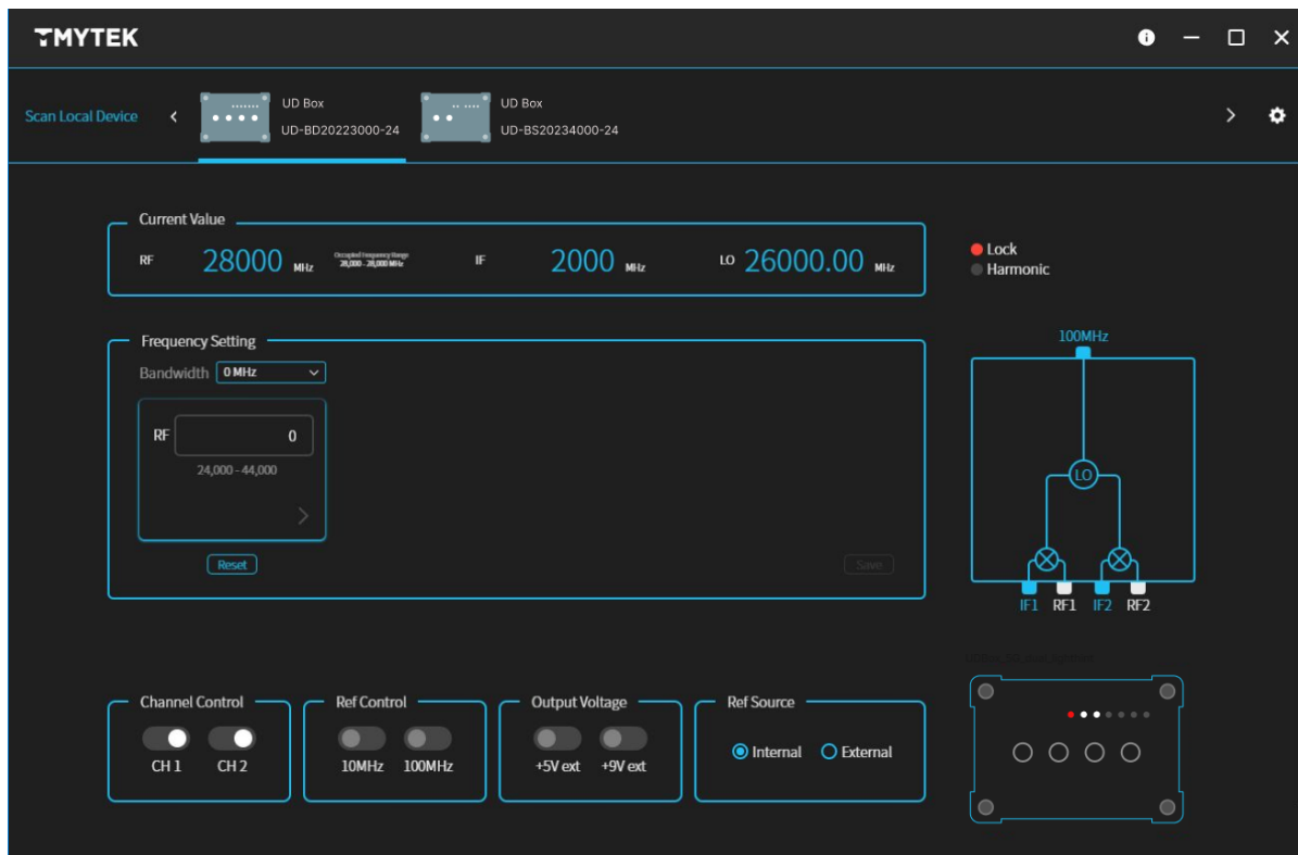
Figure 4. Controlling UD Box 5G using TMXLAB Kit
